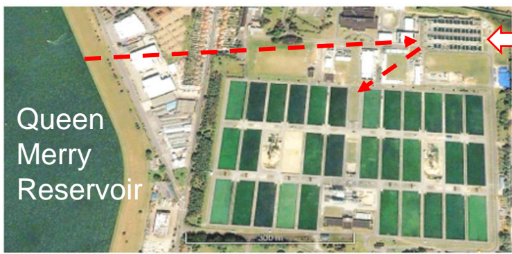
Biological roughing filter without chemical.
