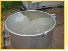
There were extremely small particles like as colloidal particles in case of small turbidity, like as less than 20 NTU. The rapid settling of turbid matters was observed within 4 hrs. However, a large portion of turbidity did not decrease.
