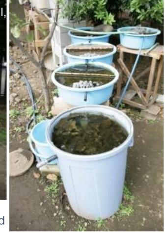
There are sedimentation tank, several gravel filter, and slow sand filter. Polluted water turns to safe and reliable water quality.
