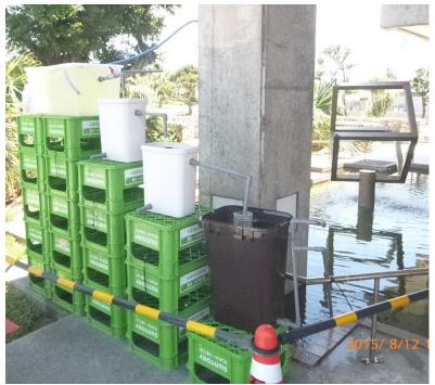
Filter rate can be measured using a cup and is regulated by a cock.
