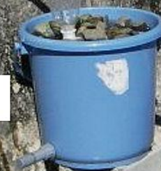
Up-flow roughing filter using gravels.
