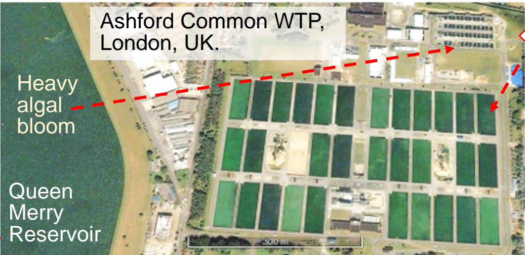
SSF 32 filters. 100mx35m
