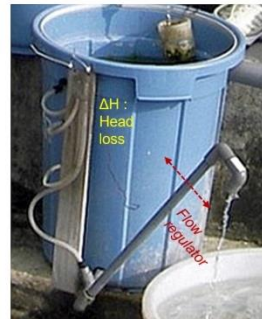
Fig. 8-5. Clog indicator is calculated with head loss and velocity.
