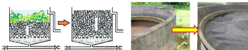
Fig. 16-8. Top up small stone in URF, March 2017
