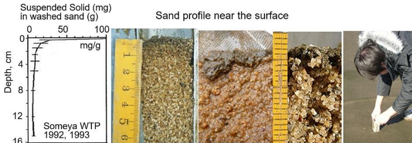
Fig. 7-1. Thin active layer is only at the top of sand layer.
