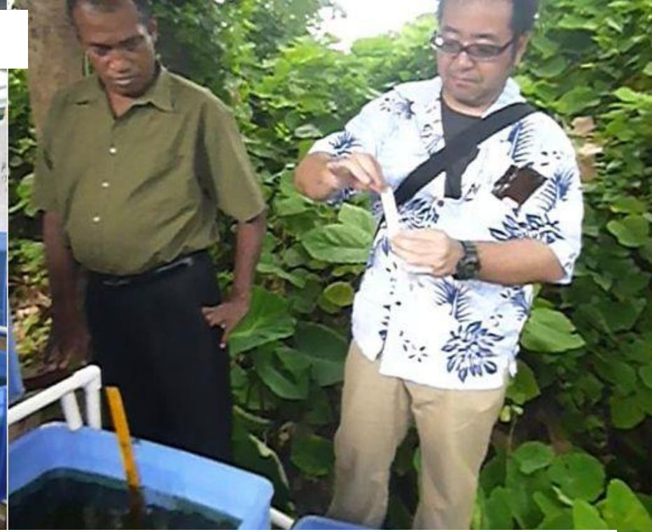
We can check the safety by use of bacteria test paper.
