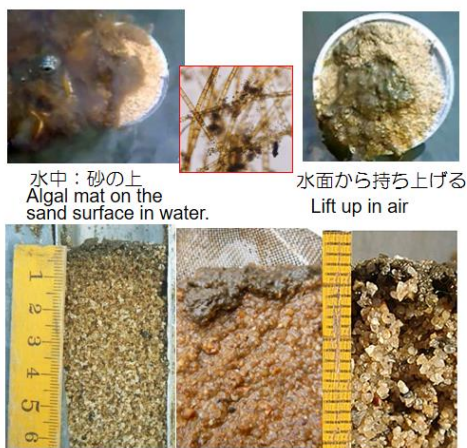
図 19-3 生物群集にやさしい維持管理をするなら砂層は汚れない Sand beneath the surface in water is clean. When the supernatant water drain off, the trapped SS releases and drops into sand layer.
