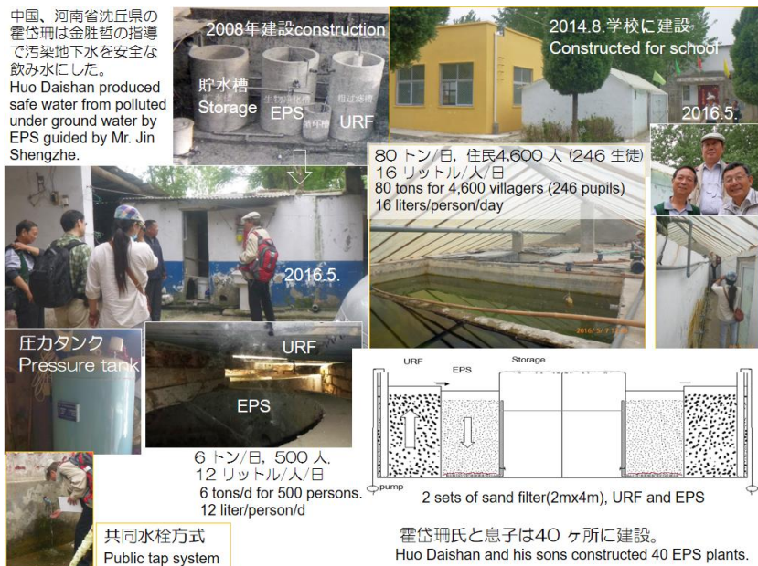
図 35-4 河南省の地下水汚染で癌村に生物浄化法で安全な水を供給 Huo Daishan constructed 40 EPS plants for villagers to supply safe drinking water from the heavily contaminated ground water.
